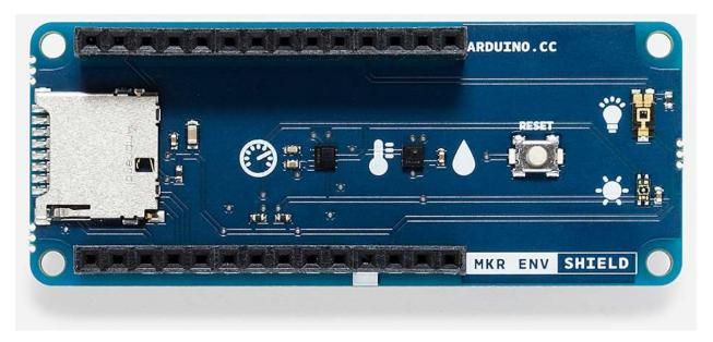
The first sensor on the left is an LPS22HB and measures atmospheric pressure; the next one is an HTS221 and measures temperature and humidity, next is the reset button that has been replicated on the shield to allow you to reset the MKR board below. The top sensor on the right is a TEMT6000 and measures the Lux of the ambient. The last sensor, just below the Lux, is a VEML6075 and measures the two UV wavelengths named as A and B. This last sensor is also capable of producing the
